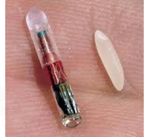
Small RFID chip, here compared to a grain of rice, is incorporated in consumer products, and implanted in pets, for identification purposes
